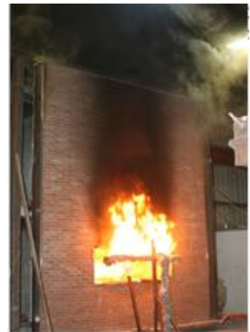
Photo 1. NFPA 285 testing of brick veneer cavity wall with foam plastic and a combustible WRB on gypsum sheathing over steel frame wall construction
